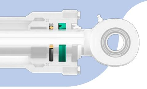
Rod and buffer seals maintain sealing contact in a sliding motion between the cylinder head and the piston rod. A rod sealing system can consist of a rod seal and a buffer seal or a rod seal only. For heavy duty applications, rod sealing systems typically consist of a combination of both seal types, whereas the buffer seal is arranged between the rod seal and the piston in the cylinder head.
